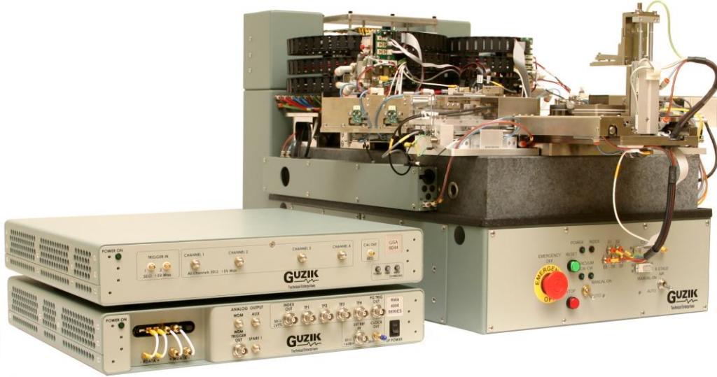
Figure 3. Complete RWA Test System with GSA 6044
